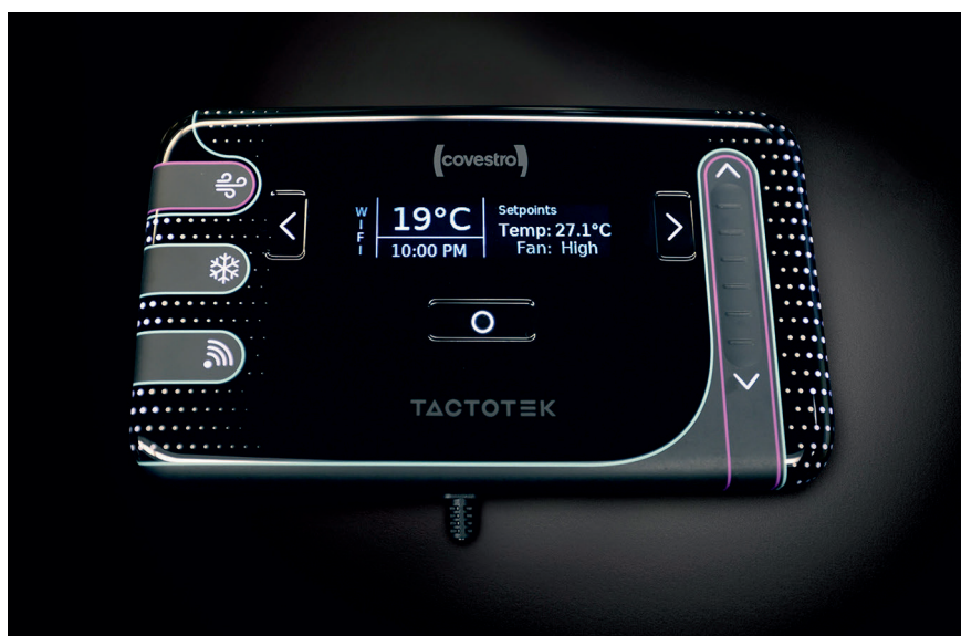
Fig. 2. In addition to capacitive touch control functions and an OLED display, the Nighthawk demonstrator, which is only 3.5 mm thick, also integrates functional lighting elements and ambient lighting. © Covestro
